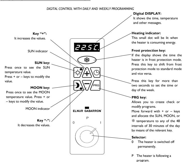
RXE Plus models have built in an electronic thermostat with a sensibility of 0.1  $^{\circ}$ C. It is possible to set temperatures with an accuracy of 0.5  $^{\circ}$ C.
