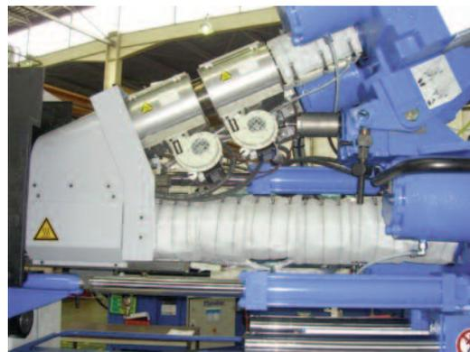
Insulation mattresses on cylinder of a injection molding machine
