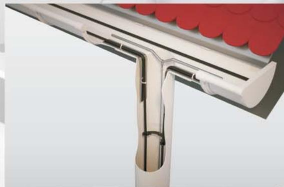
Protection of the heating cable against "wear-through"
